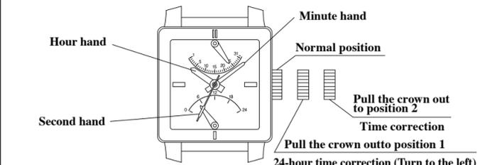
※If the crown is a screw-lock type, loosen the screw before operating the crown. When operations have been completed, retighten the screw.
