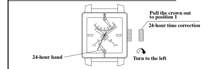
The 24-hour hand enables the setting of the time for another time zone. The 24-hour time setting can be made in 1-hour increments to enable use of the dual time function.
